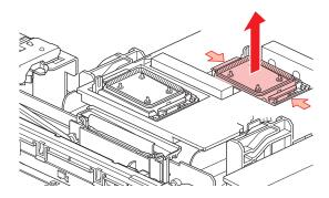
[When using Sb ink and TP ink] Rinse the cap with the mesh side facing downward in a container filled with maintenance liquid. Remove, then wipe clean the resin part thoroughly.
