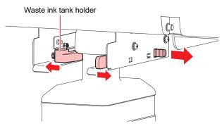
(2) Hold the waste ink tank handle and pull it forward to remove it.
