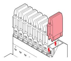
**?** Remove the ink absorber, and replace with a new one.
